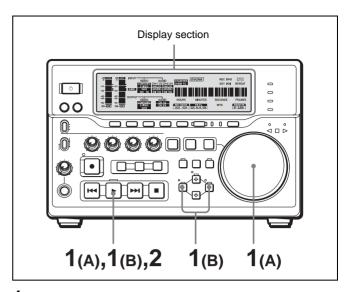
1 (A)Hold down the PLAY button, and turn the search dial in the desired direction to adjust the playback speed.
